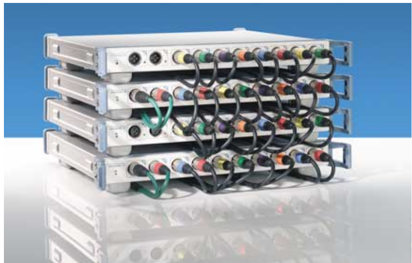
With the Audio Switcher UPZ, up to 128 input and 128 output channels can be cascaded
